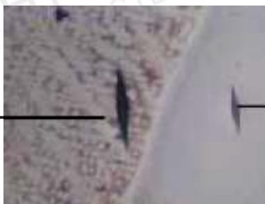
Hardness impression is a PS-98 Matrix 58Rc
